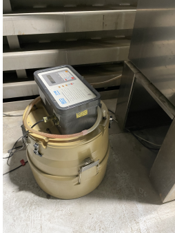
(a) Isco 3700 Portable Sampler used for sampling PI.
