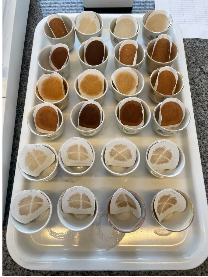
Figure 3.4: Some of the filters in the crucibles after incineration in the furnace at 550 °C.
