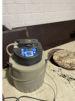
(b) Isco 6712 full-size portable sampler used for sampling PE.
