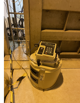
(c) Sigma 900 Composite Sampler from Hach used for sampling SE.
