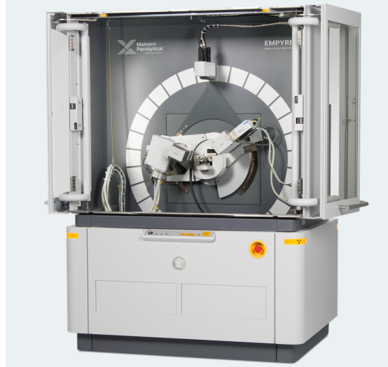
Figure 3.4: Empyrean, Serie III, Malvern Panalytical XRD Machine [86]
