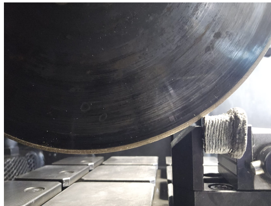
Figure 3.9: Cutting blade and the Mo sample
