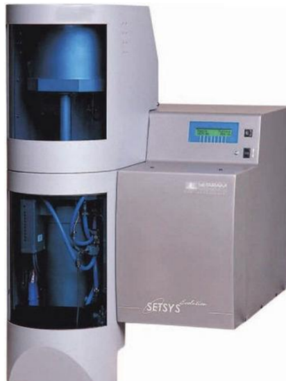
Figure 3.16: SETSYS Evolution TMA Machine
