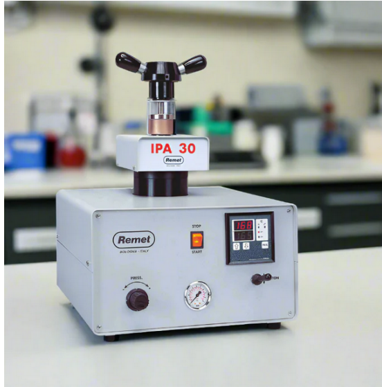
Figure 3.11: Remet IPA 30 Hot Mounting Machine [91]
