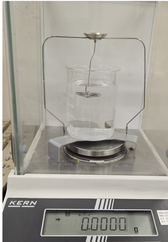
Figure 3.10: Archimedes Density Analysis Setup
