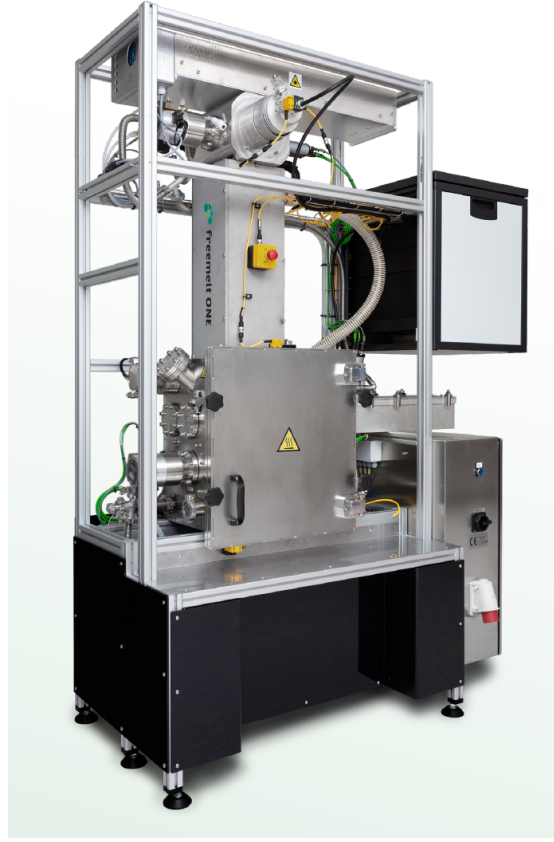
Figure 3.6: Freemelt ONE PBF-EB Machine [45]
