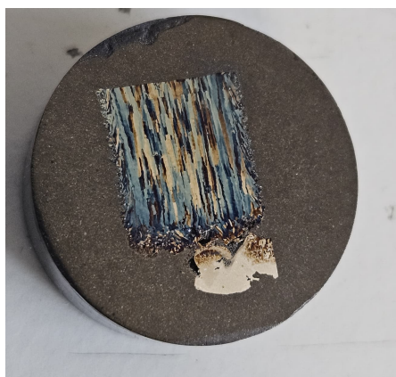
Figure 3.15: Samples after being etched by HF solution
