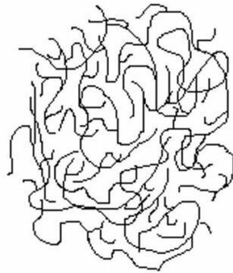
Figure 1.3 Semi-crystalline polymers (left) contain sections of ordered structure, while amorphous polymers (right) have an unorganized structure.
