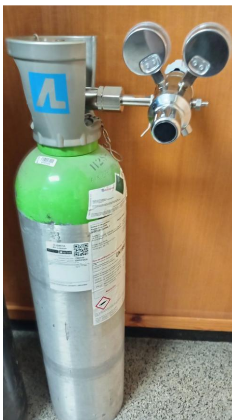
Figure 13: Gas cylinder of hydrogen sulphide with a concentration of 3000 ppm \text{H}_2\text{S}/\text{N}_2 .
