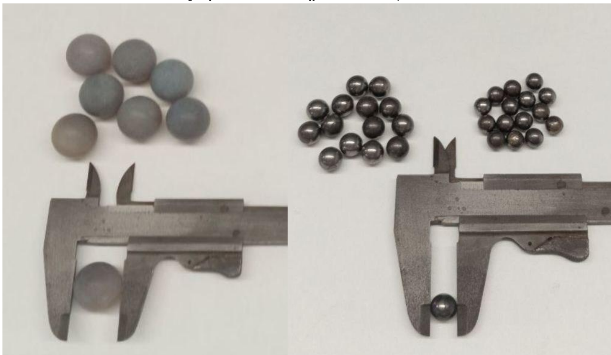
Figure 6 & 7: Comparison of ball sizes used in the ball milling experiment on the left large balls, on the right mixed-ball size.
