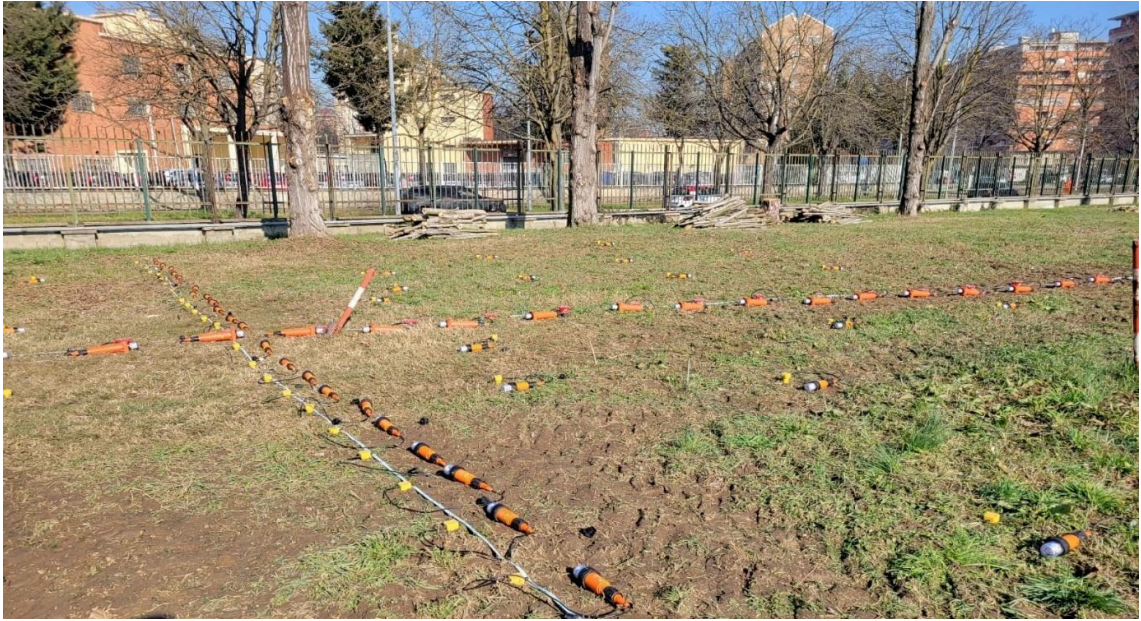
Figure 3-4 Field setup of the receiver array at the CNR test site.
