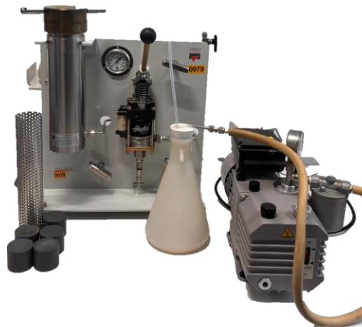
Figure 10. Actual saturation setup used in the laboratory, including the water flask, the empty trap and the vacuum pump forming the evacuation line.
