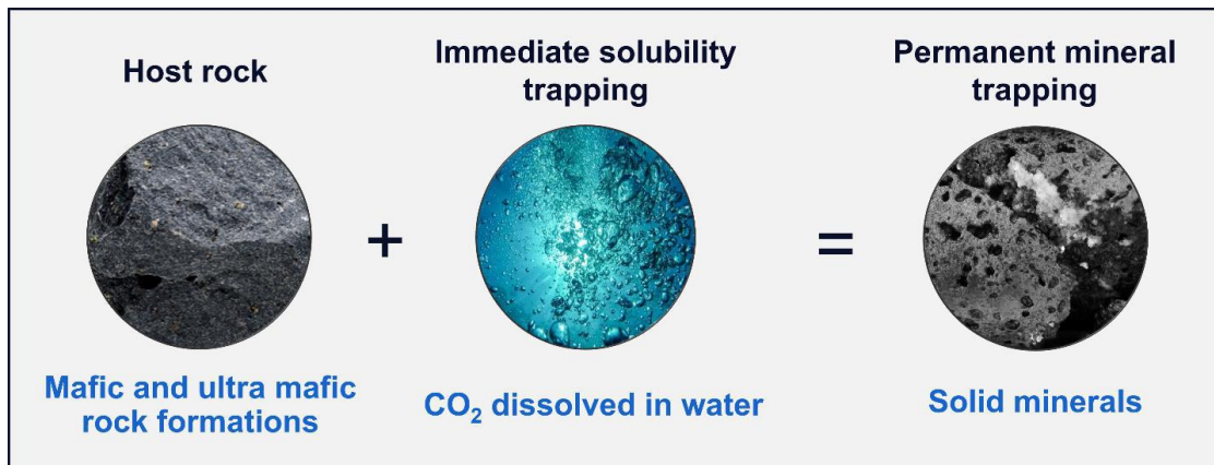
Figure 3 Simplified diagram of in-situ carbon mineralization (Ye, Li, Wang, & Zhao, 2025)
