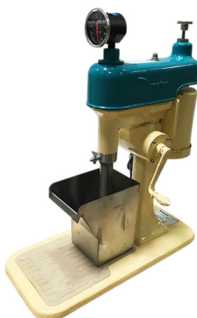
Figure 4: An image of Denver Type Flotation Machine (911Metallurgist, 2016).
