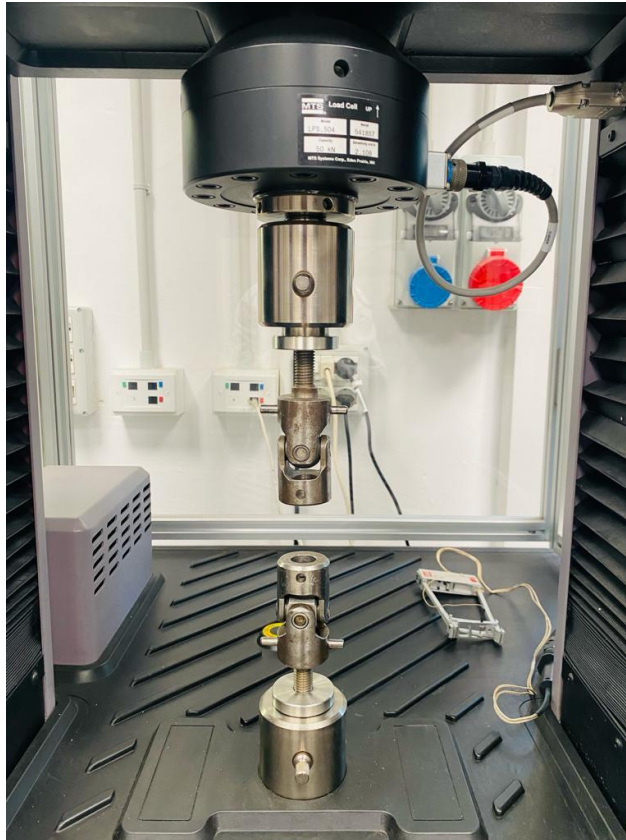
Figure 3.7: MTS Tensile Tester, model LPS.504 with a capacity of 50 kN
