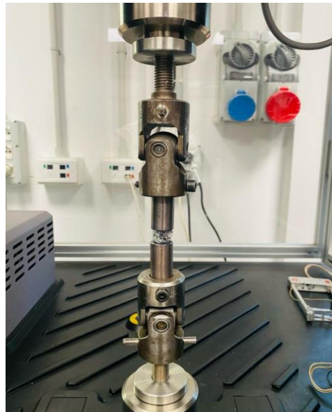
Figure 3.11: MTS tensile tester with Aluminum sandwich foam sample mounted in the holder with adhesive bonding
