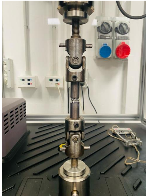
Figure 3.10: MTS tensile tester with Aluminum foam sample mounted in the holder with adhesive bonding
