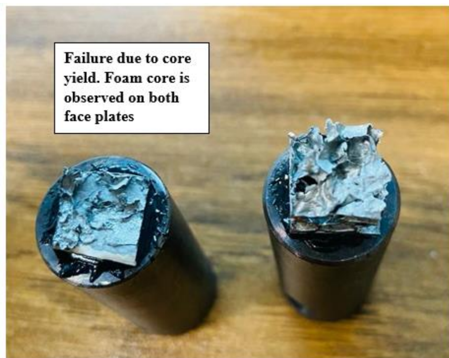
Figure 5.5: Failure of foam core of the sandwich panel SD Al6016 Al Zn
