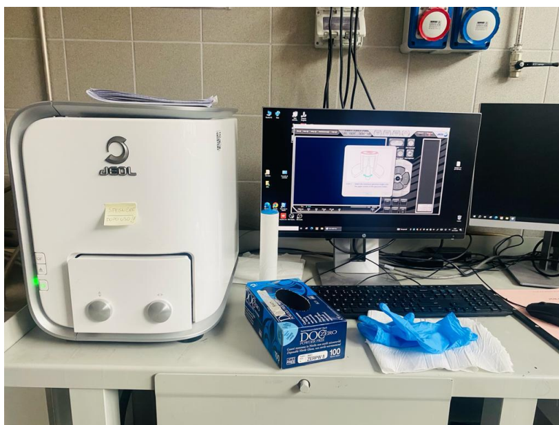
Figure 3.13: JEOL JCM-6000Plus electron microscope
