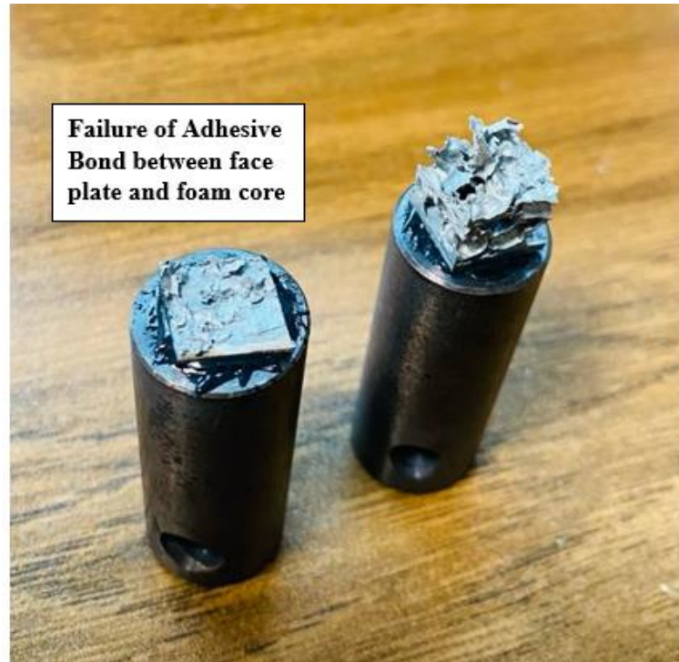
Figure 5.3: Failure of adhesive bond between aluminum face plate and foam core of the sandwich panel SD Al6016 Al 2 Zn
