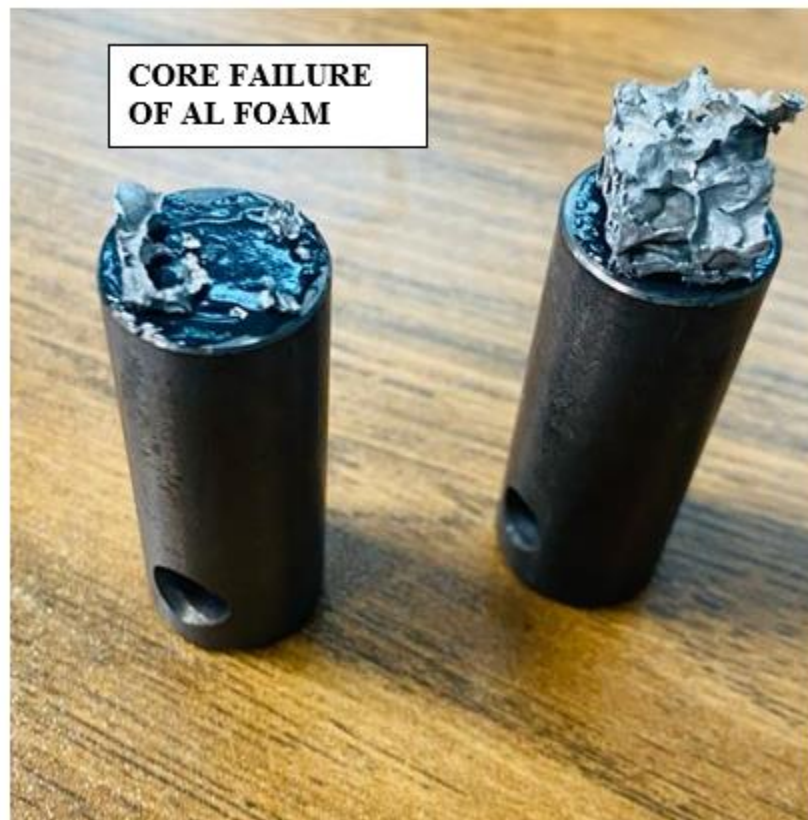
Figure 5.1: Aluminum foam core failure mode
