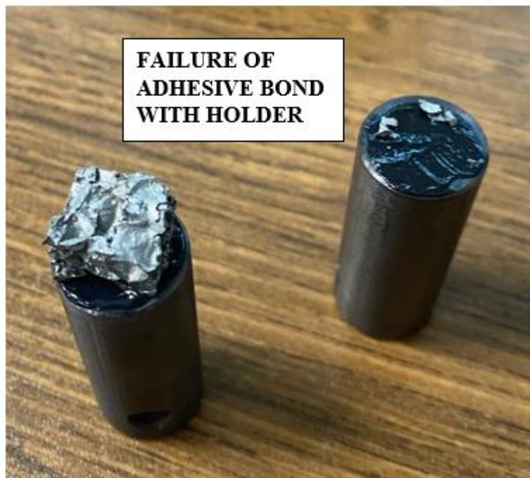
Figure 5.2: Failure mode showing failure of adhesive bond between Al foam and holder
