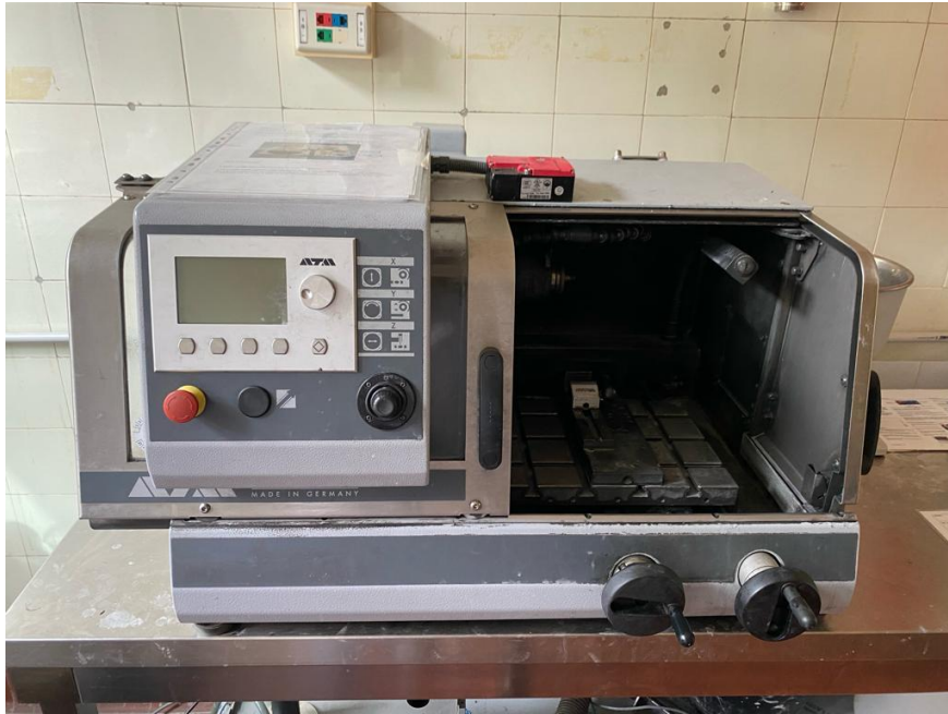
Figure 3.8: QATM auto cut off machine for sizing and cutting metal samples
