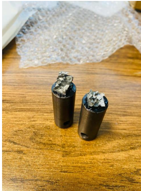
Figure 3.12: Ruptured sample of aluminum sandwich foam SD Al6016 Al Zn
