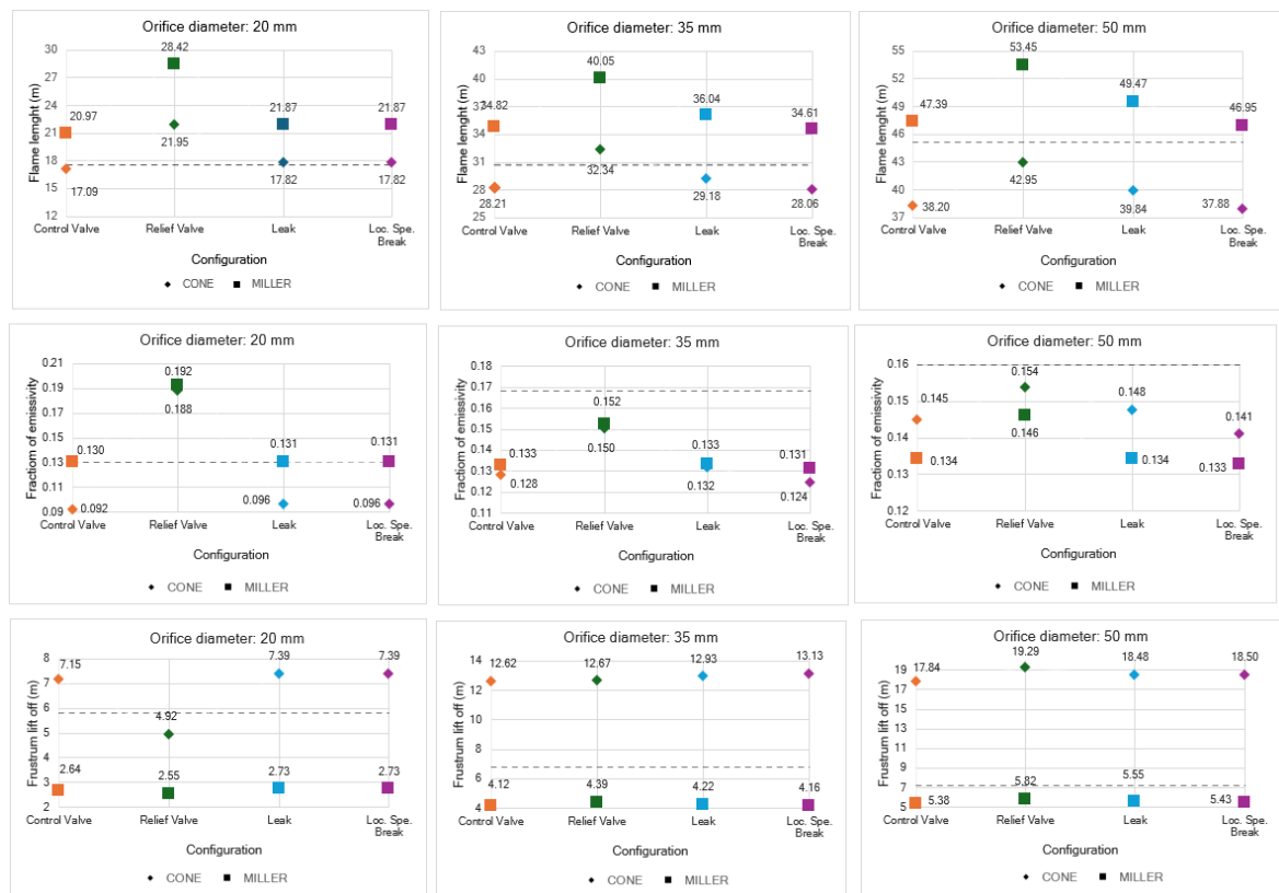
Figure 22. Flame length, fraction of emissivity and frustum lift off distance simulated for 20 mm, 35 mm, 50 mm orifice diameters with four different configurations: a horizontal pressure vessel with a control valve (orange; 1), relief valve (green; 2) or leak (light blue; 3); or a long pipeline with a specific location of the break (purple; 4). The
