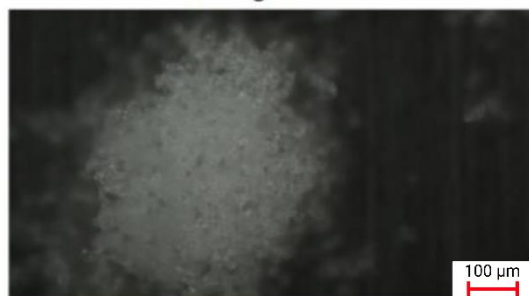
Figure 44. Unexpanded TEPs under optical microscope (no adhesive matrix)
