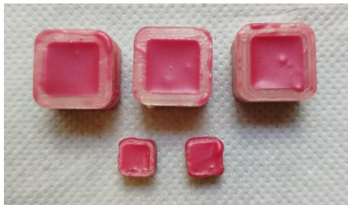
Figure 24. Cast-cured Specimens Inside the Hydrosoluble Molds
