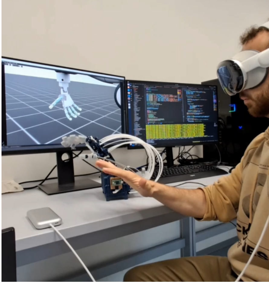
Figure 3.3: AVP teleoperation system and Adapt Hand sim2real setup for recording
