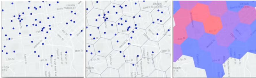
Figure 2.10: The maps depict the process of bucketing points with H3: cars in a city; cars in hexagons; and hexagons shaded by number of cars. Picture from note 11.
