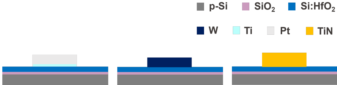
Figure 3.1: MFIS stacks layout. From left to right: Ti+Pt, W and TiN gate metal
