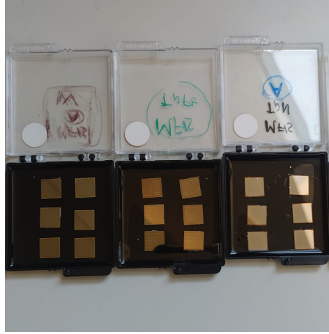
Figure 3.2: Chips with MFIS stacks. From left to right: W, Ti+Pt and TiN gate metal. Per each metal: 3 chips with and 3 chips without post-metalization annealing
