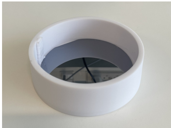
Figure C.1: 3D-printed circular holder hosting a Si wafer with diameter 100 mm: liquid PDMS is ready to be poured on top.
