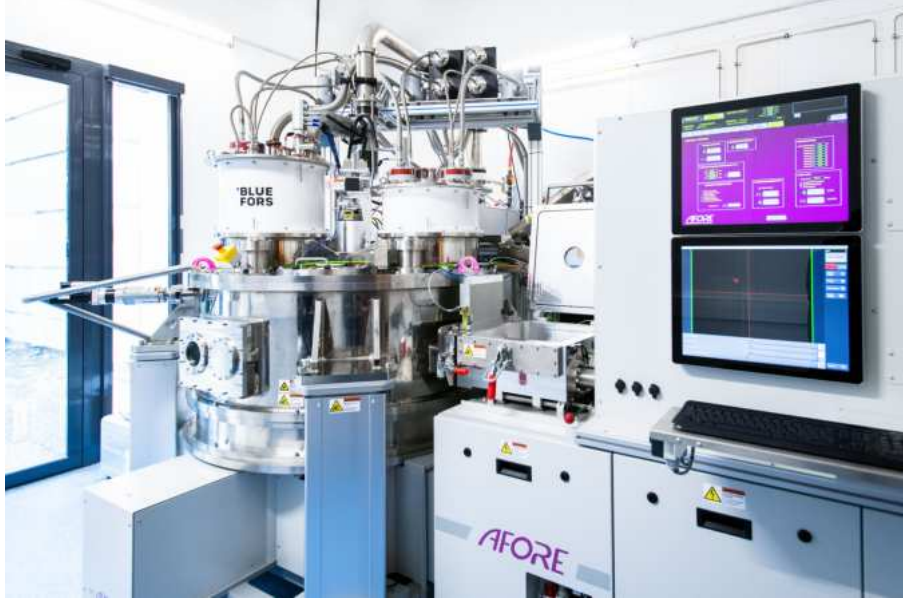
Figure 4.1: Wafer Cryogenic Prober used to acquire the CSDs data.
