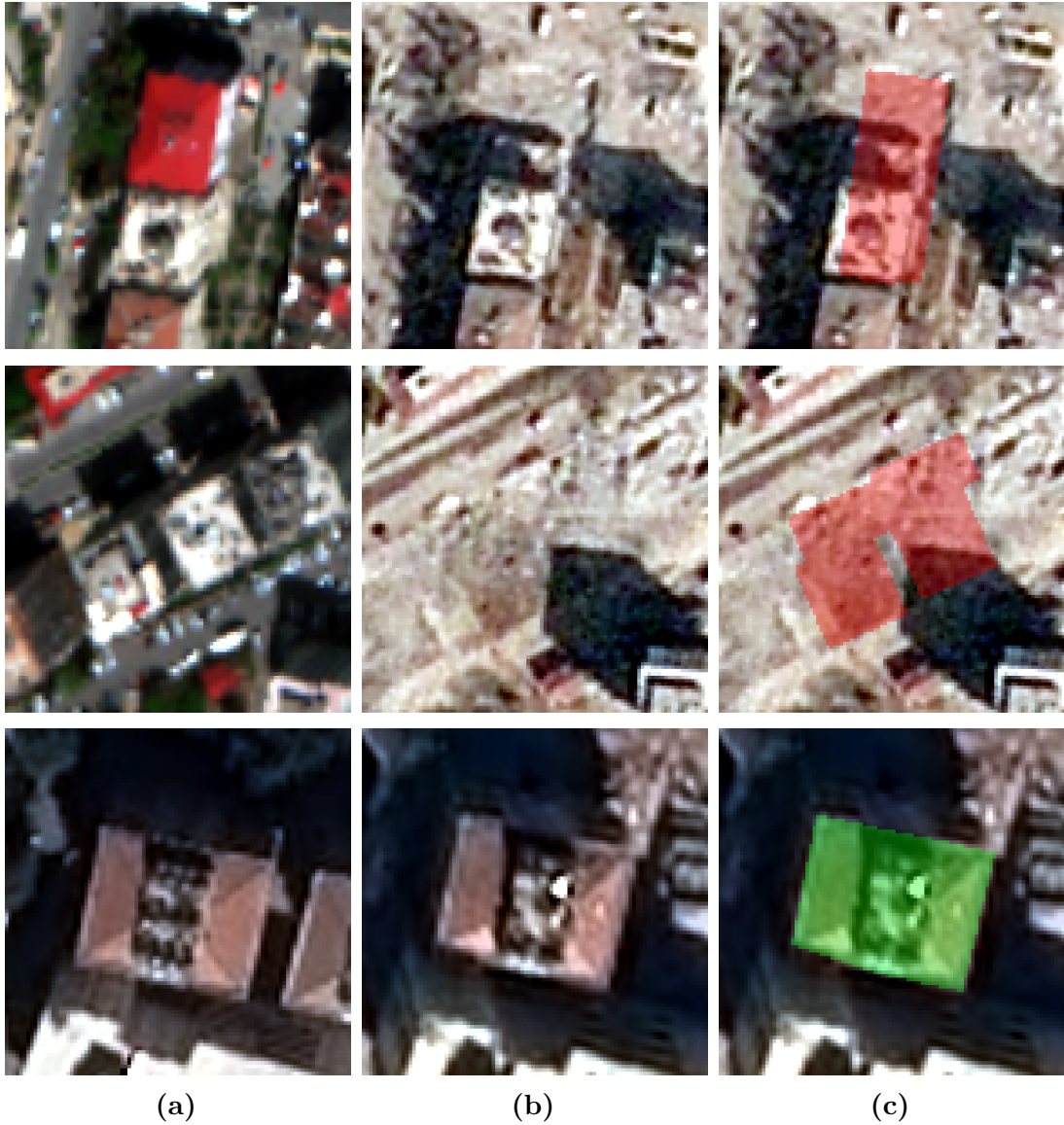
Figure 5.2: (a) Pre-event; (b) post-event; (c) ground-truth mask. In the project, ground-truth masks are encoded as 0=undamaged, 1=damaged, 255=background; in images above the mask is visualized as an overlay on the post-event image (red=damaged, green=undamaged).
