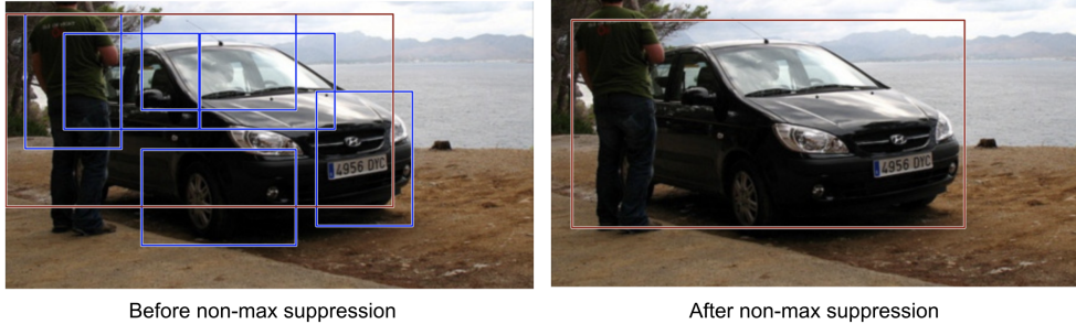
Figure 2.15: Multiple bounding boxes detect the car in the image. After non-maximum suppression, only the best remains and the rest are ignored as they have large overlaps with the selected one [33].
