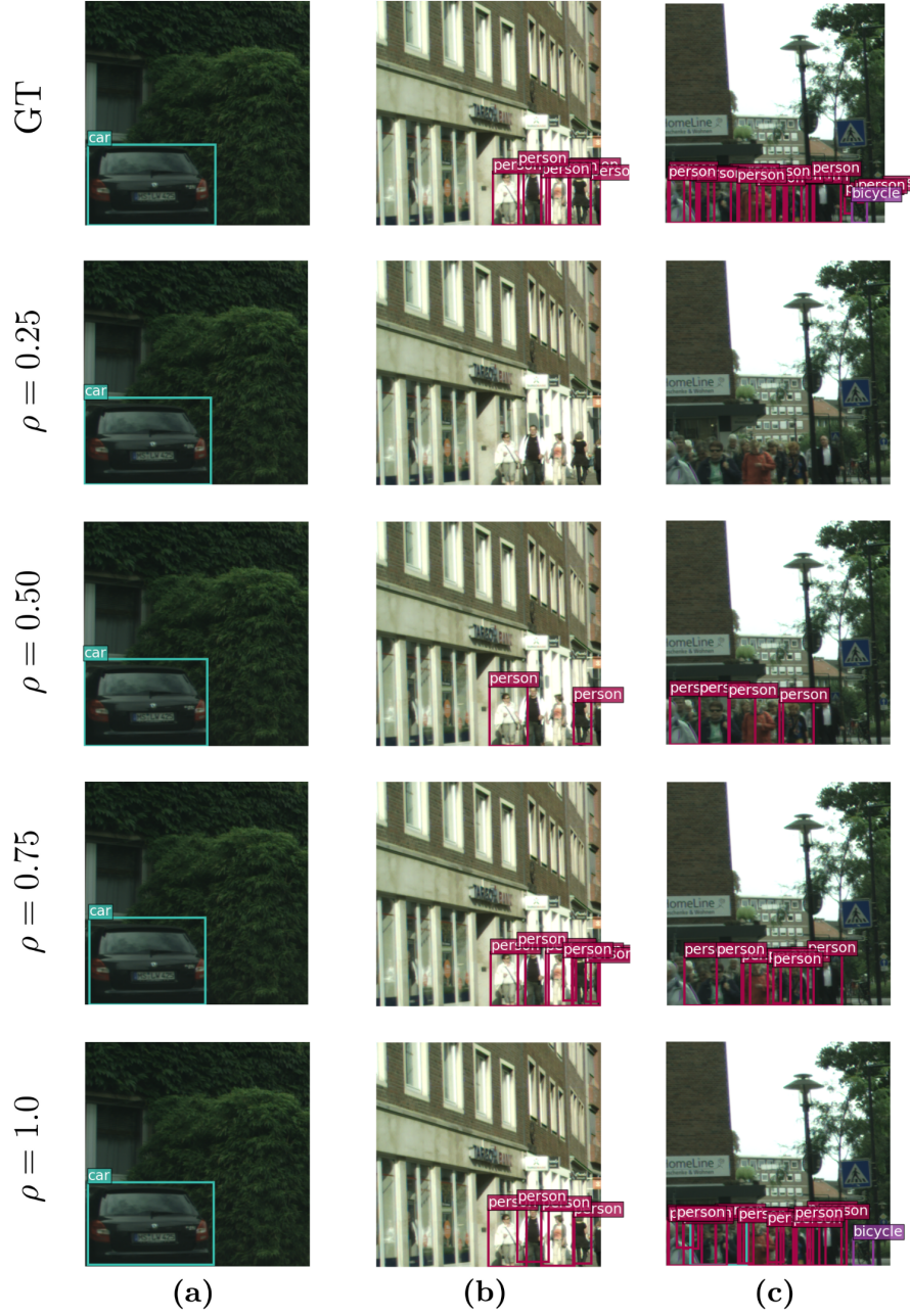
Figure 5.1: Qualitative predictions of the slimmable model in Static Mode at different slimming ratios \rho \in \{0.25, 0.50, 0.75, 1.0\} . Each column shows a representative image with ground truth (GT) on the first row and model predictions below. (a) Example with a single, clearly visible object. (b) Moderately dense and well lit scene. (c) Crowded scene with multiple objects.
