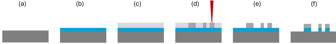
Figure 27: Preliminary simplified process for Nb patterning on \text{SiO}_2 . (a) \text{SiO}_2 on substrate. (b) Sputtered Nb thin film. (c) Spin-coat negative e-beam resist. (d) E-beam exposure to write the pattern. (e) Resist development. (f) Nb RIE etching to form the Nb features.
