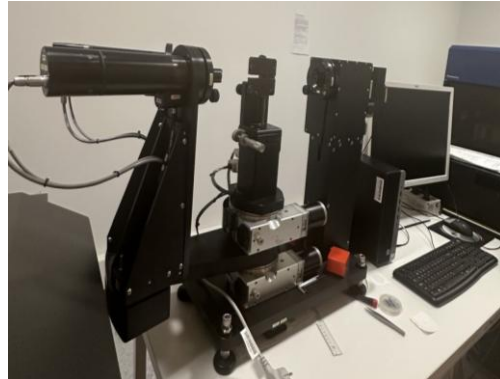
Fig. 14. (a) Fabricated 1D PhC on a 2-inch fused silica wafer. (b) Woollam VASE Spectroscopic Ellipsometer.
