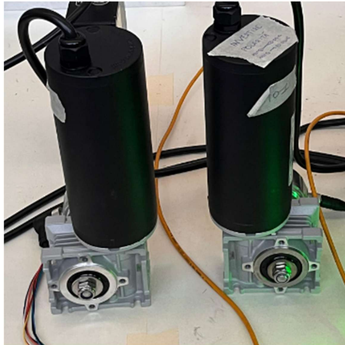
Figure 21: Motors coupled with reducers
