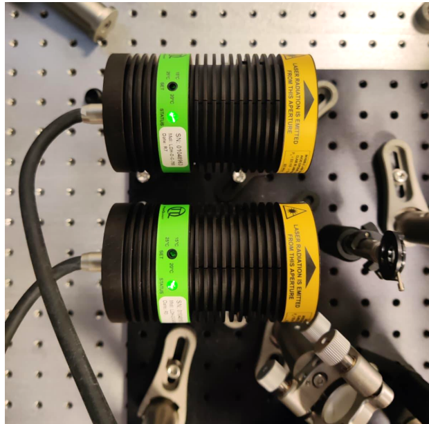
Figure 14. Two examples of the laser diodes used for pump–probe measurements.
