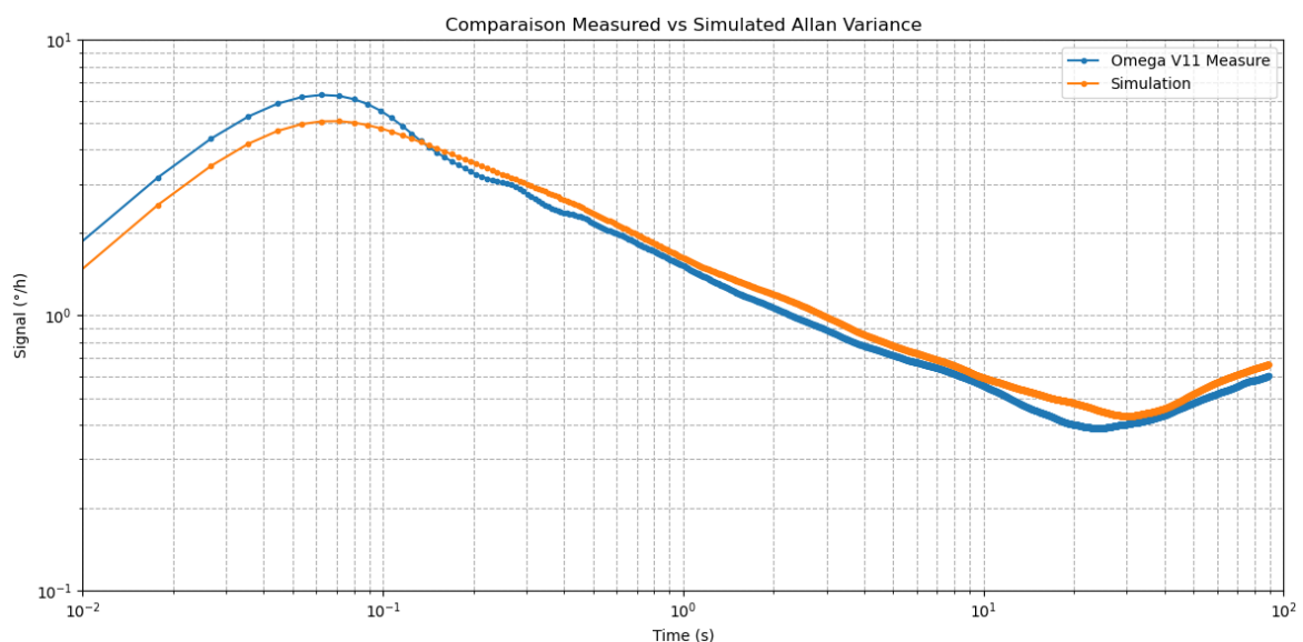
Figure 22: Allan Variance of simulated (artificially modified) and generated signals.
