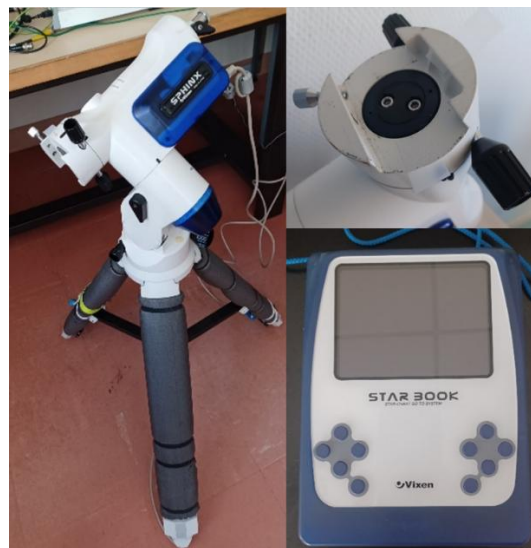
Figure 32: Image of the telescope mount in use, left. Top right, a zoomed-in view of the gyroscope's grip area. Bottom right, an image of the STARBOOK in use with the mount.
