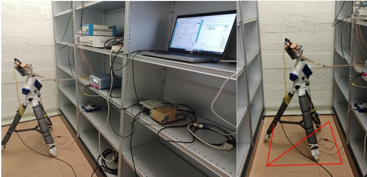
Figure 53: North-Finding experiment set up in the basement of an ONERA building. On the left, a complete view of the experiment. On the right, a zoom on the telescope mount with the construction lines on the ground to orient the mount relative to geographic North.
