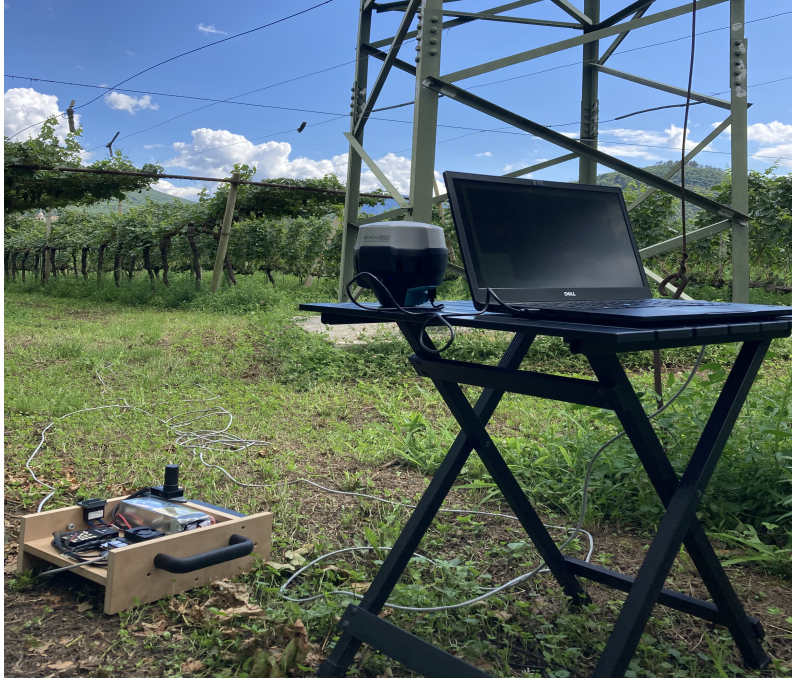
Figure 3.5: Setup during a field test on transmission tower
