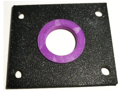
Figure 125 Gear carriage top panel with 3-D printed baffle installed (in purple)
