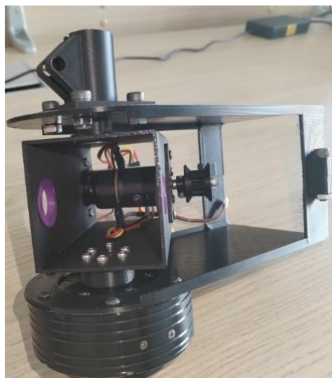
Figure 126 Partially assembled prototype with Joint 4 connections clearly visible
