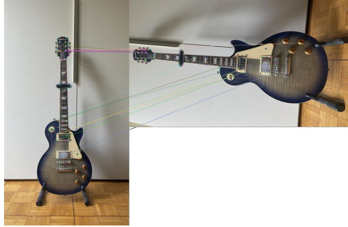
Figure 6.1: Example of feature extraction and matching via ORB.
