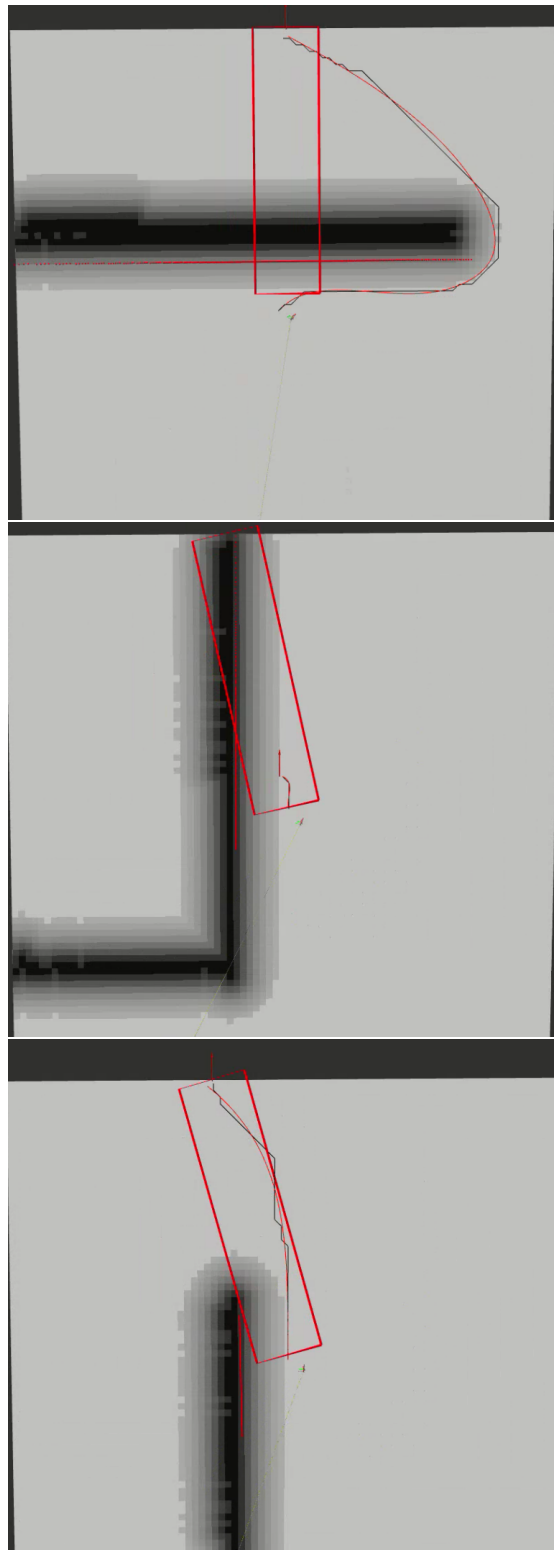
Figure 7.16: Drone simulation in World 2 with new parameters - RViz view - Collision Avoidance
