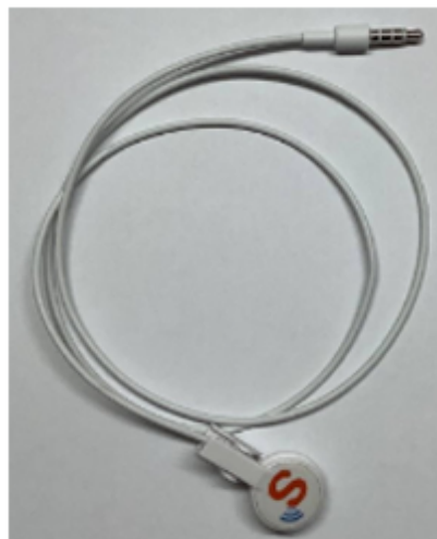
Figure 14: Shimmer3 GSR+ Unit SR48-3-0 Optical pulse clip
