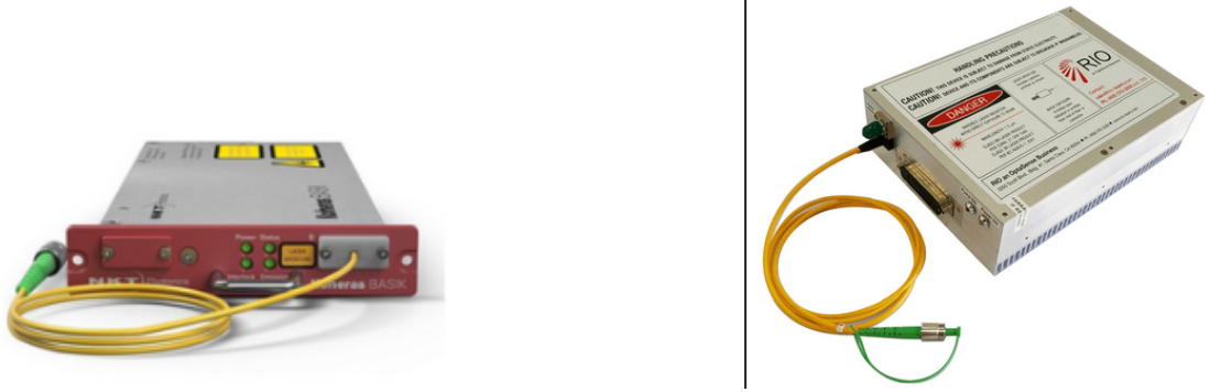
Figure 5.26: The two types of lasers used in our setup : a narrow-linewidth fiber laser manufactured by NKT as a sensing laser, and a diode laser manufactured by RIO as a quantum laser.
