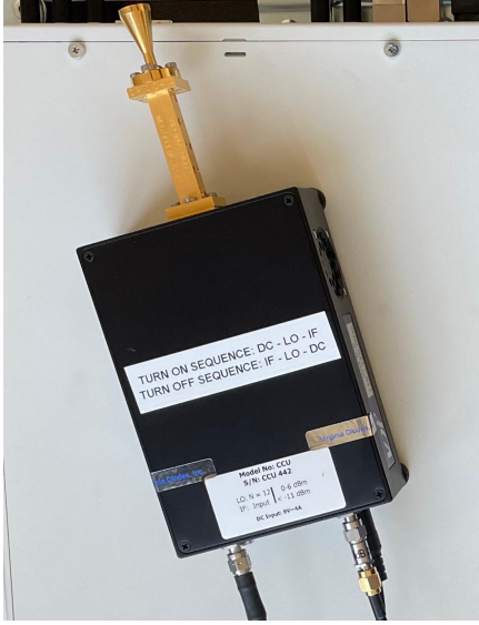
(a) VDI WR-6.5 upconverter used in the transmission chain (TX).
