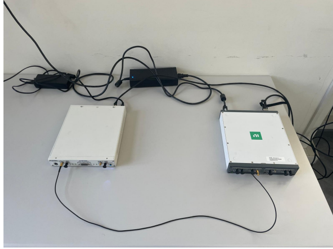
Figure 7.6: Laboratory setup for coaxial cable transmission. USRP X310 is connected to USRP X410 via coaxial cable.
