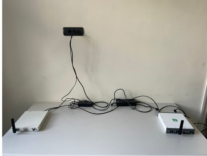
Figure 7.9: Laboratory setup for wireless transmission with antennas. TX and RX are placed at a fixed distance.
