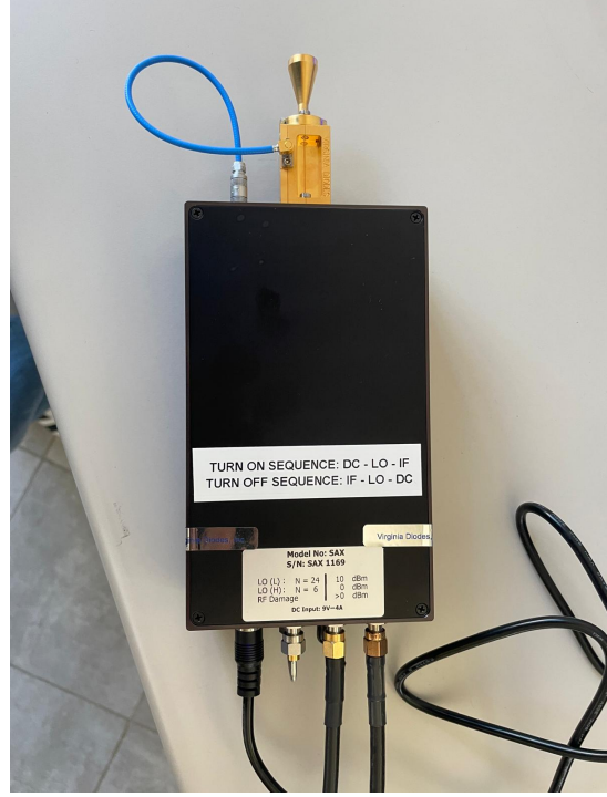
(b) VDI WR-6.5 downconverter used in the reception chain (RX).
