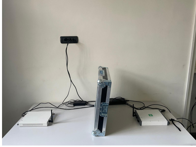
Figure 7.12: Setup for antenna transmission with an obstacle to introduce attenuation and multipath effects.
