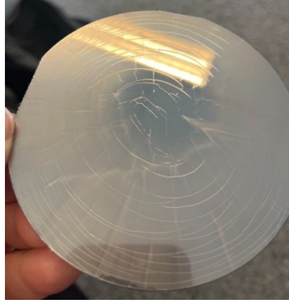
Figure 4.8: Cracks in Mo sputtered film on silicon oxide/PLA substrate.
