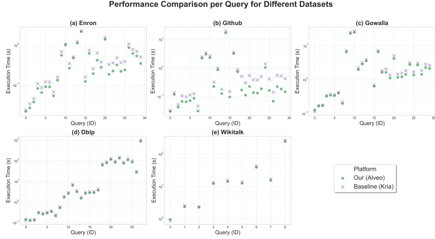
Figure 5.2: Comparison of execution time for each query for all datasets between 512-bit HBM accelerator and 128-bit DDR4 baseline accelerator.
