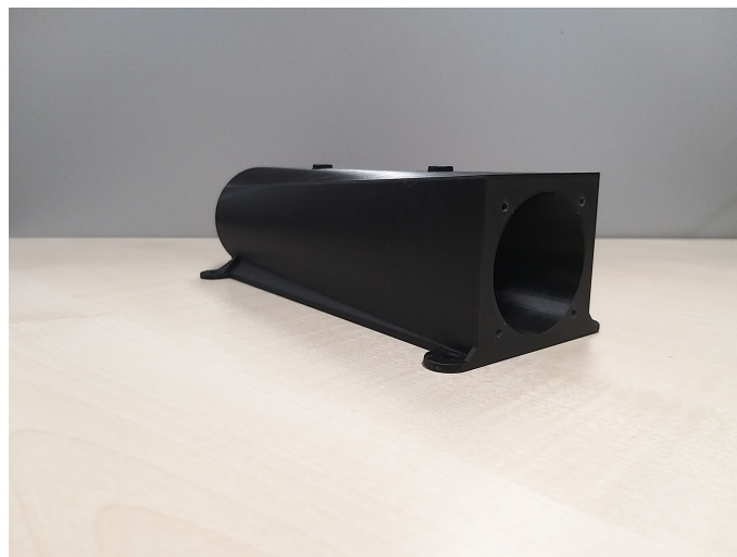
Fig. 3.4: 3D printed Venturi, first prototype. here is shown the Venturi tube from the front part where is visible the inlet but also the thread available to test the fan in a free environment.
