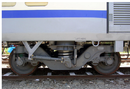
Figure 27: Main components of the axlebox-arm suspension system (left) and example of its realization in a railway bogie.
