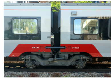
Figure 13: Example of a Jacobs bogie
