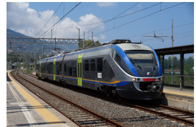
Figure 3: Ale501-Le220-Ale502 train, commonly known as 'Minuetto'; these employ railcars. They are also classified as Electric Multiple Units: often the distinction between trains containing railcars and EMUs is not clear cut.
