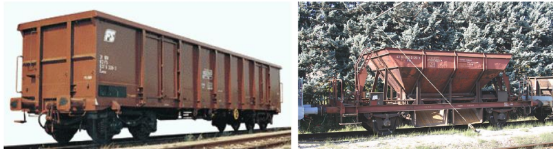
Figure 6: Examples of freight cars: Left: standard open freight car Right: hopper freight car
