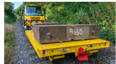
Figure 7: Trailers are typically adopted when whole freight cars are not required
