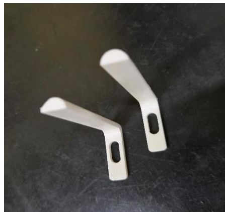
Figure 4.11: Physically realized stopper component fabricated using PLA material.
