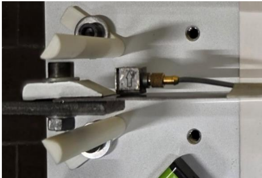
Figure 4.9: Close-up view detailing the gap between the beam tip mass and the semi-cylindrical stopper.
