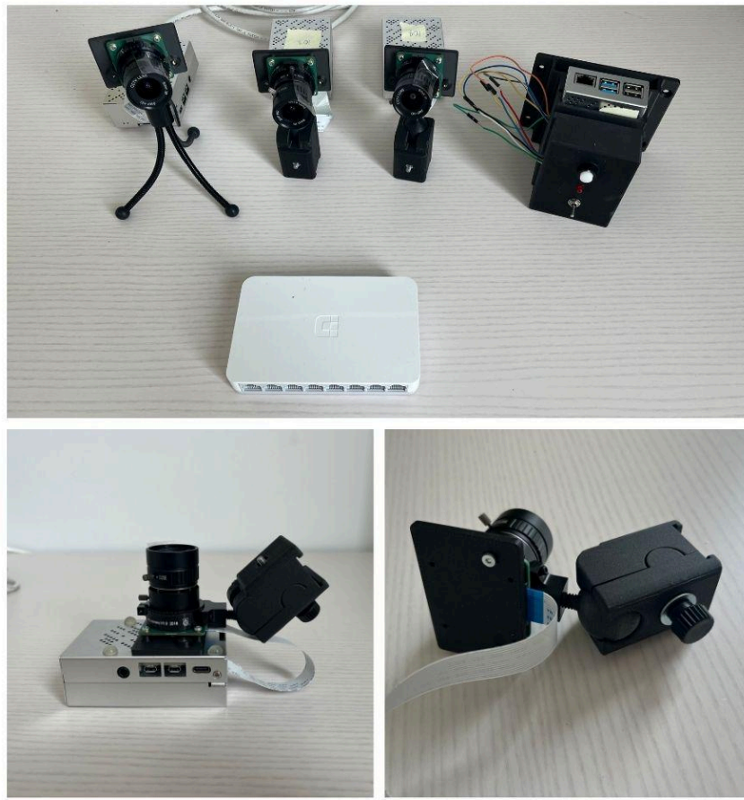
Figure 8 - Cameras and Raspberry Pi setup
