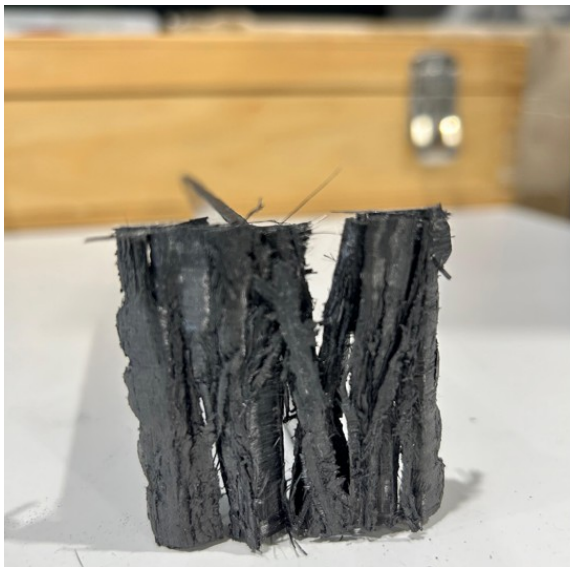
Figure 4.40: From left to right, (A) Bottom part of quasi-static CF-PC coupon. (B) CF-PC in the testing bench.
