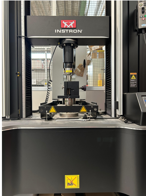
Figure 4.36: 300 [kN] Instron 6800 Series Universal Testing Machine setup.
