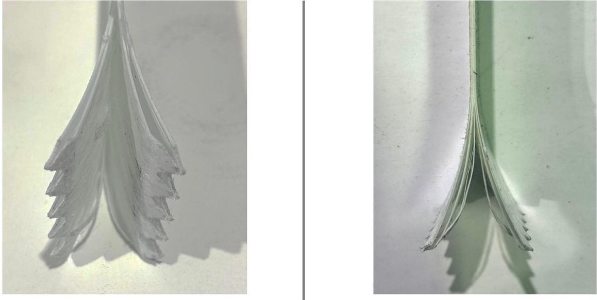
Figure 4.23: GF-PP Flat coupons after Crashworthiness Splaying test, delamination in multiple layers can be observed.
