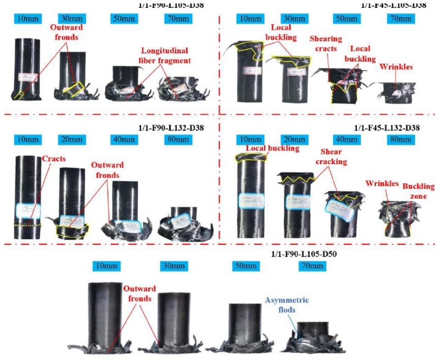
Figure 2.7: Crashworthiness test performed in tube specimens of different diameters. [14]
