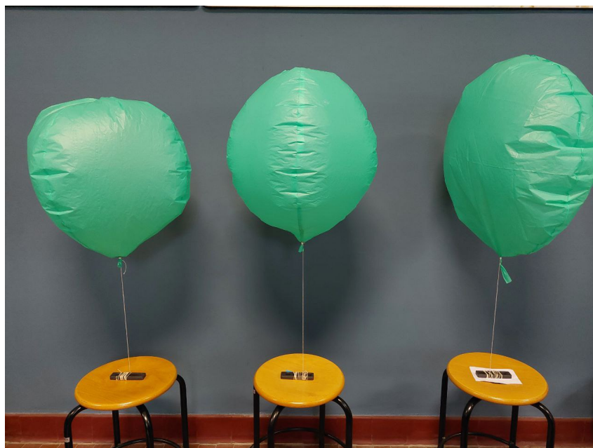
Figure 5.14: Helium retention test setup: the three balloon configurations (double-neck, top cap and Grabo sample) tied to a ballast of 200 g each. The balloons were periodically weighed together with the ballast to evaluate gas leakage over time.
