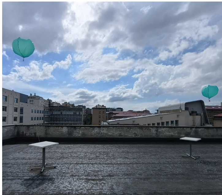
Figure 5.17: Tethered radiosondes on the roof of the Politecnico. This photo captures the moment just after the rainfall, when the decrease in wind allowed the balloons to return to a nearly vertical position.
