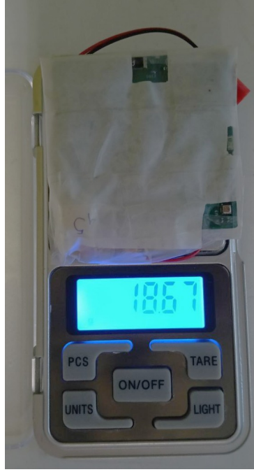
Figure 5.16: Weighting phase of the radiosonde system using a precision balance. The PCB is connected to a 450 mAh battery, and the protective adhesive tape leaves free the ventilation hole of the sensor (visible in the bottom right corner).
