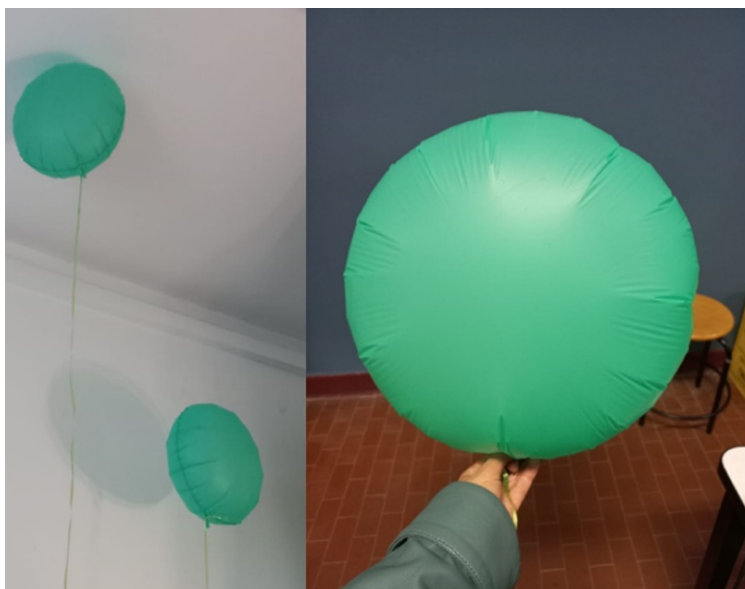
Figure 5.1: First production test of Mater-Bi balloons using two circular sheets, developed in collaboration with Grabo Srl.
