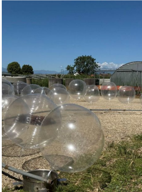
Figure 6.13: Nineteen-inch Grabo Mylar balloons inflated and temporarily secured to a support pole before being attached to the probes.
