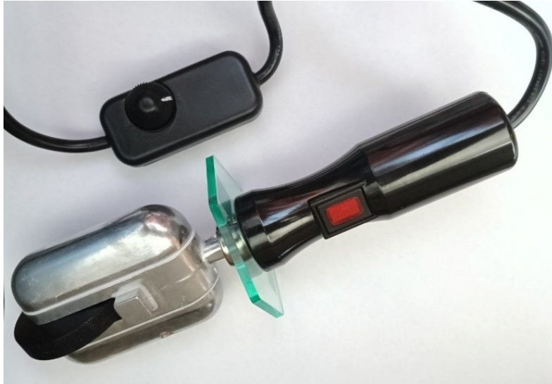
Figure 4.4: Hand-operated wheel sealer with a temperature control knob.
