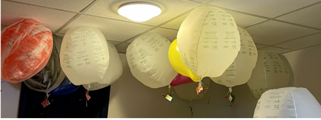
Figure 3.2: Cluster of radiosondes connected to Mater-Bi balloons, ready for launch.
