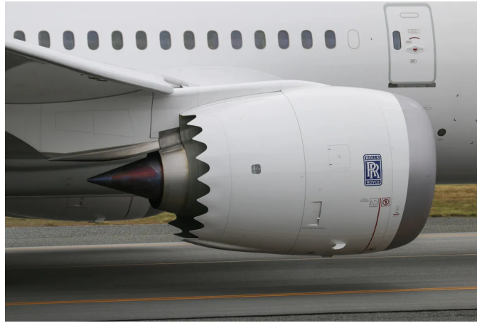
Figura 3.8: Close-up view of the Rolls-Royce Trent 1000, with its distinctive chevrons on the nacelle [17]
