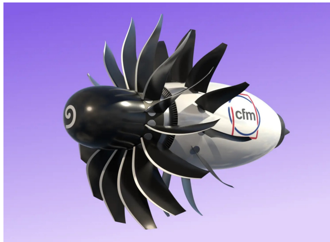
Figura 3.15: Open Fan architecture of the CFM RISE program [23]
