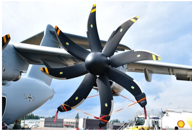
Figura 3.11: Hamilton Sundstrand A400M 17,5 ft diameter propeller system [19]
