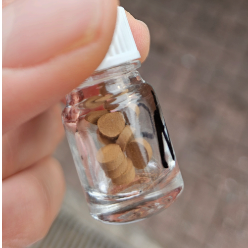
(a) Compressed Cork 2 samples stored in glass vials immediately after pressing.
