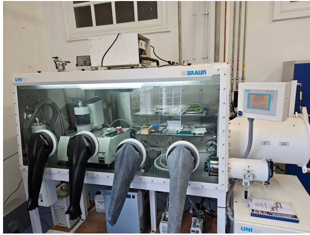
(a) Lab view: STA analyser inside the glovebox.
