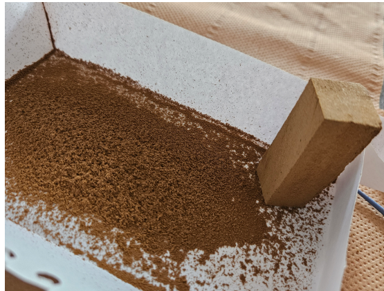
Figure 4.2: Cork 2 board slice and corresponding ground powder used for sample preparation. Powdering combined with compression allows for higher sample mass and improved contact with the crucible.
