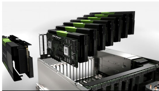
FIGURE 6.1: Example of an NVIDIA multiple GPU workstation
