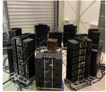
Figure 1.8: Reverberant chamber on the left vs loudspeaker array for a DFAN test on the right (source [4]).
