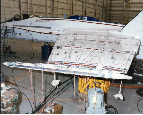
Figure 2.1: Accelerometer Setup (source [12]).
