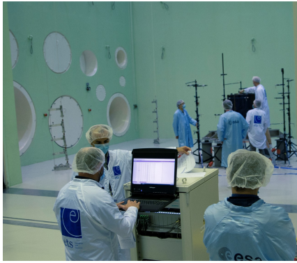
Figure 1.8: Reverberant chamber on the left vs loudspeaker array for a DFAN test on the right (source [4]).
