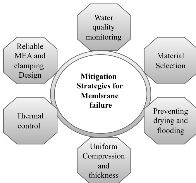
Figure 5.10: Some mitigation techniques for reducing membrane degradation and failure based on [99]
