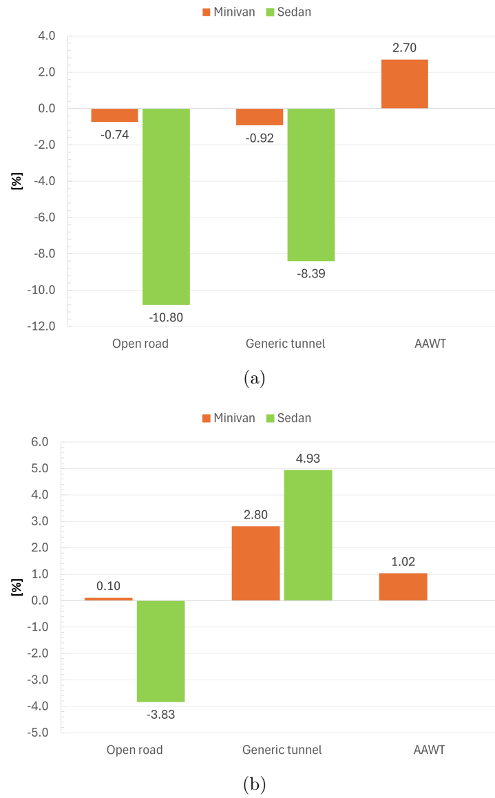
Fig. 4.2: Percentage difference between current and previous drag coefficients. a) pressure drag contribution, b) viscous drag contribution
