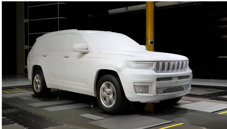
Fig. 2.8: Mock-up vehicle in the upgraded wind tunnel of Stellantis US [18]
