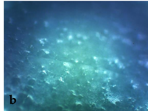
Figure 3.32. Fracture occurs after 7th cycles in (a) sample 3 and (b) sample 4
