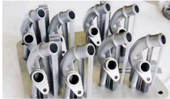
Figure 1.2. Titanium 3D printing automotive exhaust manifold adopts DMLS 3D printing [F6].
