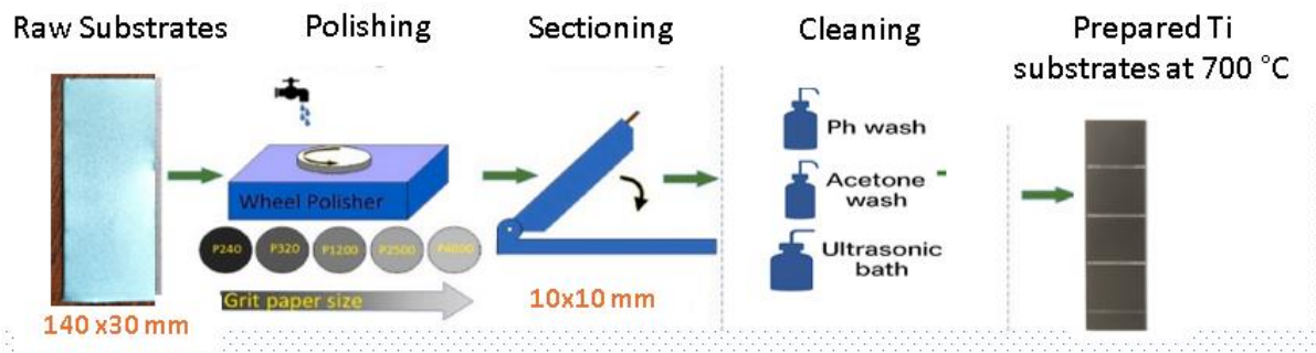
Figure 3.1. Preparation stage for Ti substrates prior to coating glass
