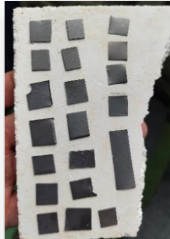
Figure 3.6. Several cut Ti substrates heat treated at 700 °C
