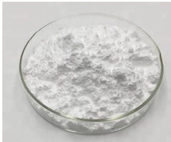
Figure 3.7. Glass powder (G1-d) after grinding
