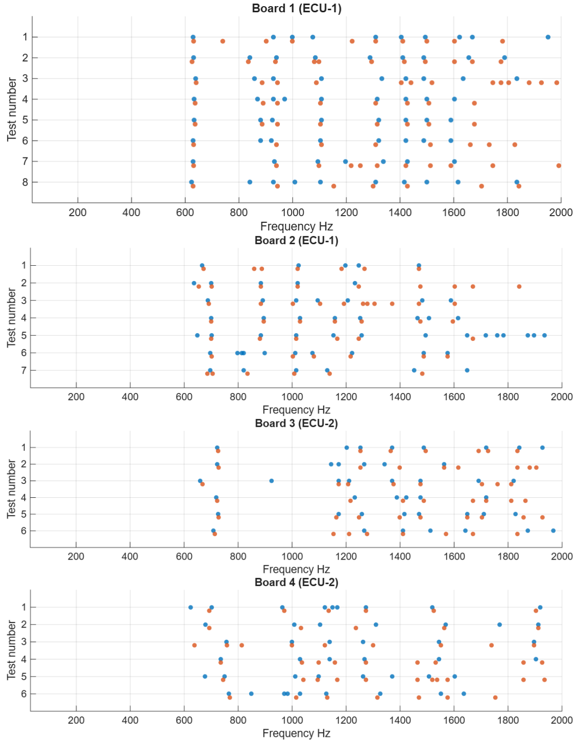
Figure 2.18: Resonance peaks identified for all the boards in all test configurations (linear scale)
