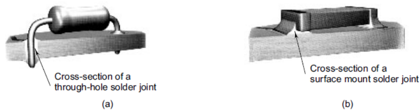
Figure 1.7: Classification of components based on attachment method: (a) through-hole component; (b) surface-mount component [2].
