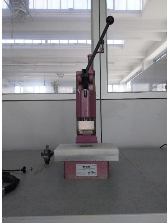
Figure 4.4.1: Instrument to cut the specimens
