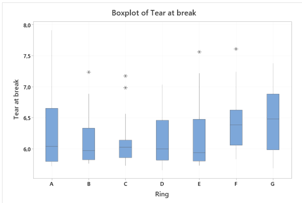
Figure 5.5.2: Boxplot of tear strength at break values grouped by the position of the ring inside the tube
