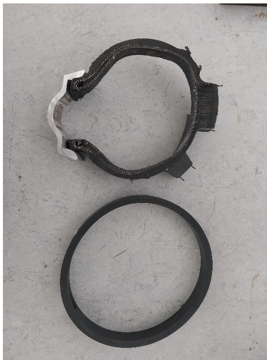
Figure 4.2.2: Section of a motorcycle enduro tyre (top) and ring used for laboratory tests (bottom)
