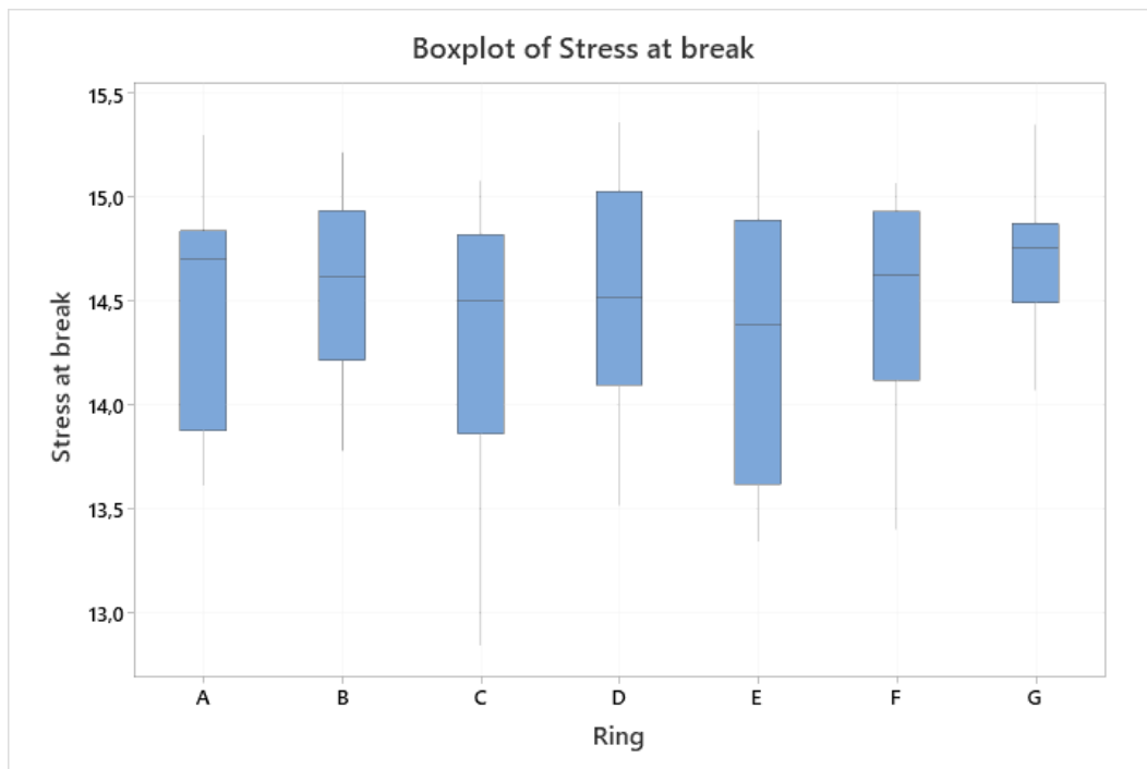
Figure 5.3.2: Boxplot of stress at break values grouped by the position of the ring inside the tube
