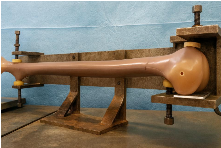
Figure 2.2-3. Left femur placed on a level surface supported by the clamping ring to mark the sagittal plane. Credits to [33].
