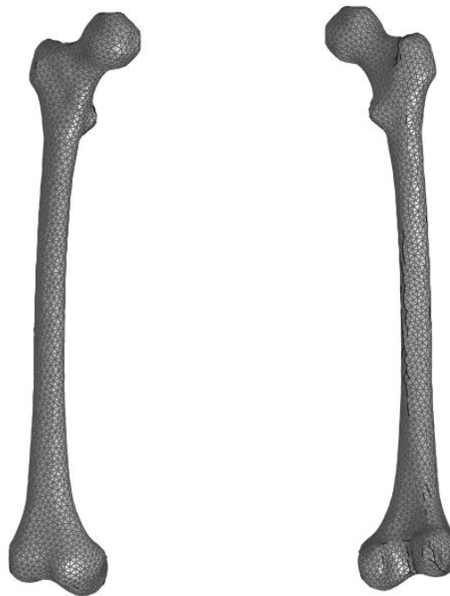
Figure 2.3-21. Before the actual meshing process in Hypermesh 2019, femur #3154 has been isotropically remeshed in MeshLab to enhance the quality of the STL obtained from 3DSlicer and prevent further complications during the realization of the 3D mesh. The resulting femoral surface is a single, continuous component composed of triangular elements.
