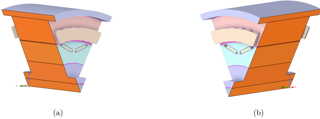
Figure 3.6: Periodic boundary conditions: (a) Rotational periodic boundary surface of one-eighth motor.1(b)Rotational periodic boundary surface of one-eighth motor.2
