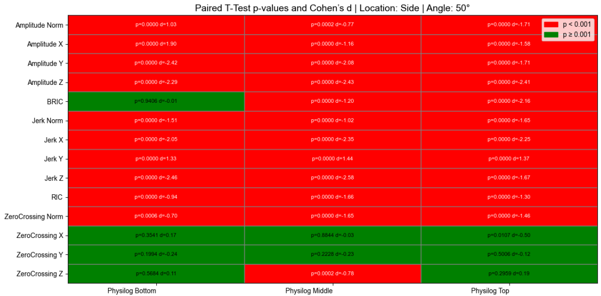
Figure 5.14: Visual summary of paired t-test results comparing the Headform reference sensor with helmet-mounted Physilog sensors (Top, Middle, Bottom) for Time-domain features, Side impact direction, 50°.
