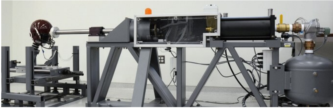
(b) Linear impactor setup [13].
