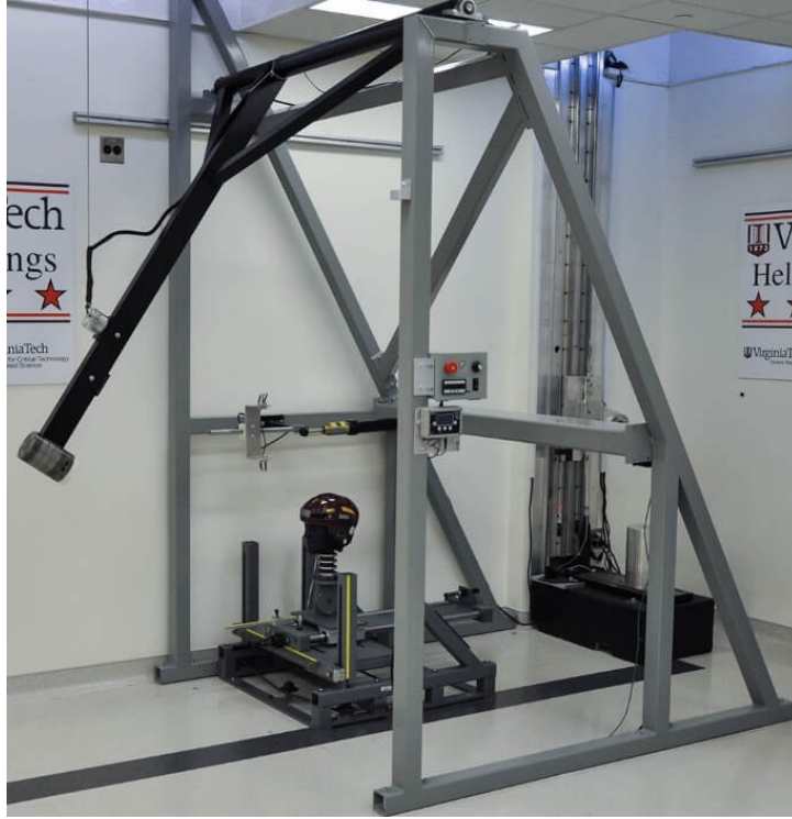
(a) Rigid pendulum impactor setup [13].
