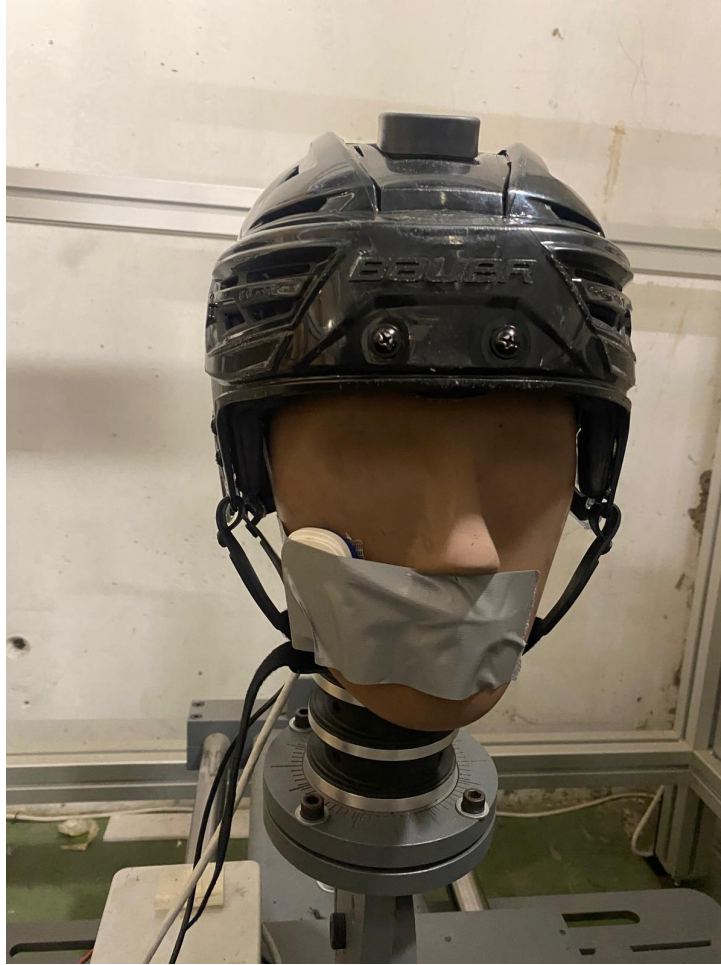
Figure A.2: Positioning of the Physilog Middle sensor on the dummy's face during trigger events.
